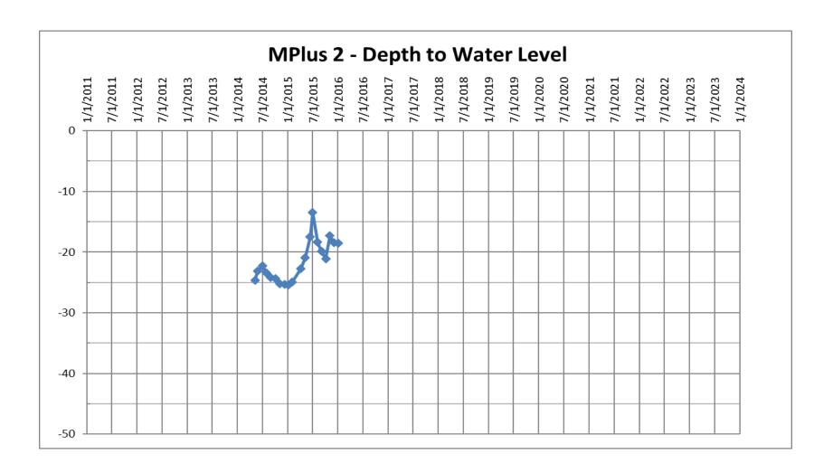
Well Designation: MPlus 2; State Well #: 309982; Well Depth: 90'; Drill Date: 1/15/2013; Screen Interval: 50-90'
