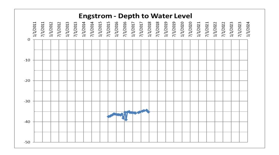
Well Designation: Engstrom; State Well #: 319220; Well Depth: 80'; Drill Date: 4/5/2013; Screen Interval: 60-80'
