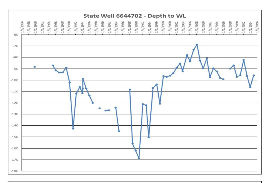
Well Designation: State Well # 6644702; Well Depth: 676'; Drill Date: 0/0/1946; Screen Interval: NA
